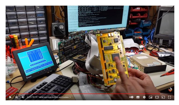
But the point is, this MFM hard drive emulator is not transferring data very quickly, and Adrian suspects that perhaps that's because the emulator was low-level formatted with a one-to-one sector interleave. Which is to say, with no sector interleaving at all. But the controller he has the emulator hooked up to needs some sector interleaving. It's not quick enough to catch the immediate next sector after reading the previous one.
