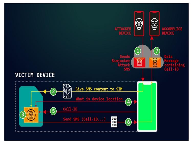
The Simjacker Attack Message could carry a complete malware/spyware payload because it contains a list of instructions that the SIM card is to execute. As software is essentially a list of instructions, and malware is 'bad' software, then this could make the Simjacker exploit the first real-life instance of spying malware sent within a SMS. Previous malware sent by SMS has been limited to sending links to malware, not the malware itself within a complete message.
